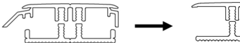
First cut the profile to the correct length. Use the slitler to cut away piece X and piece Y to obtain an expansion profile. Then use knife B to slit the profile in half. For installing, gently press the profile from one side of the rail to the other. Press against the floor.
