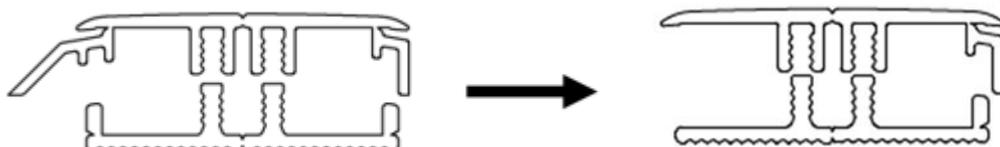
First cut the profile to the correct length. Use the slitter to cut away piece X to obtain a square nose. For installing, gently press the profile from one side of the rail to the other. Press against the floor.
