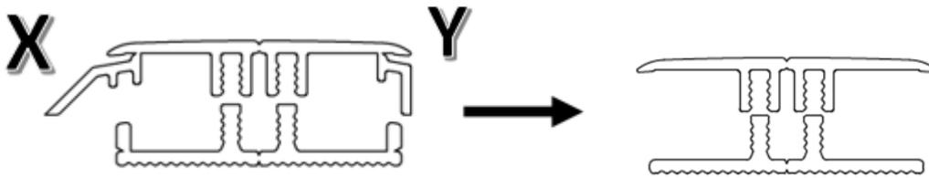
First cut the profile to the correct length. Use the slitler to cut away piece X and piece Y to obtain an expansion profile/T-molding. Remark: for easy cutting, cut both lengths before removing the 2 features. For installing, gently press the profile from one side of the rail to the other. Press against the floor.
