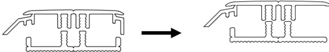
First cut the profile to the correct length. Use the slitler to cut away piece Y to obtain an adaptor profile/reducer. For installing, gently press the profile from one side of the rail to the other. Press against the floor.
